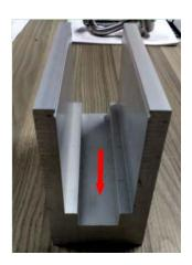
Step 2: Put L shape gasket into the channel
